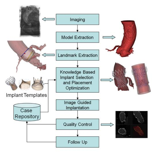
Figure. 8 Workflow and dataflow for knowledge-based implant selection and implantation support.
